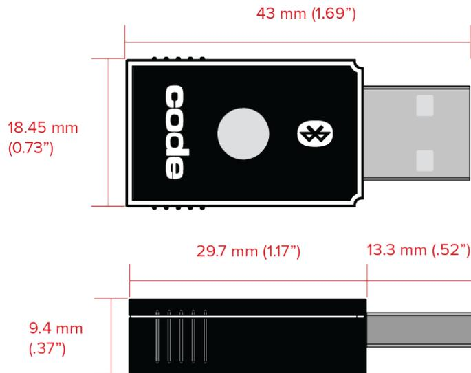
Figure 21-b CRA-BTDG27 Bluetooth Dongle Dimensions
