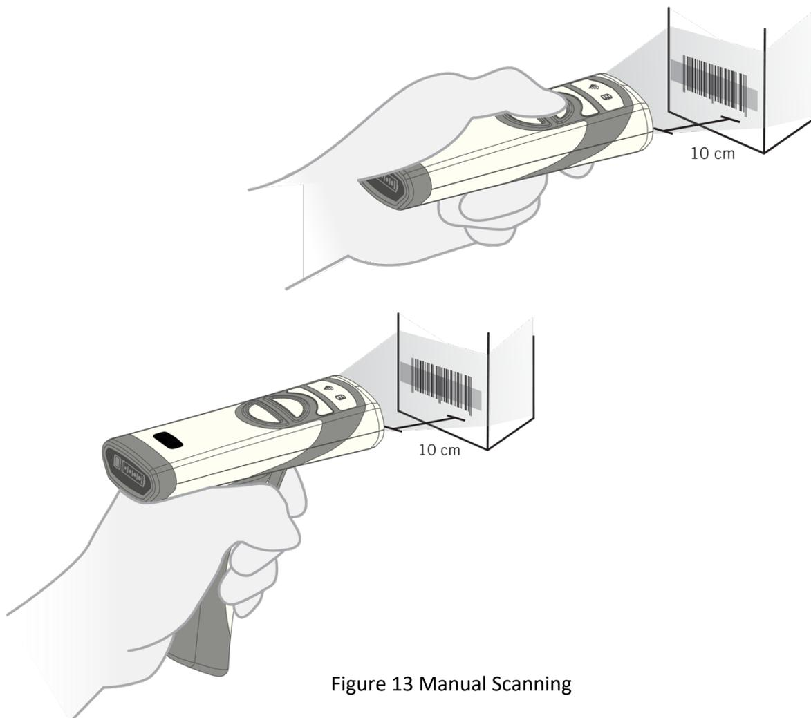
Figure 13 Manual Scanning
