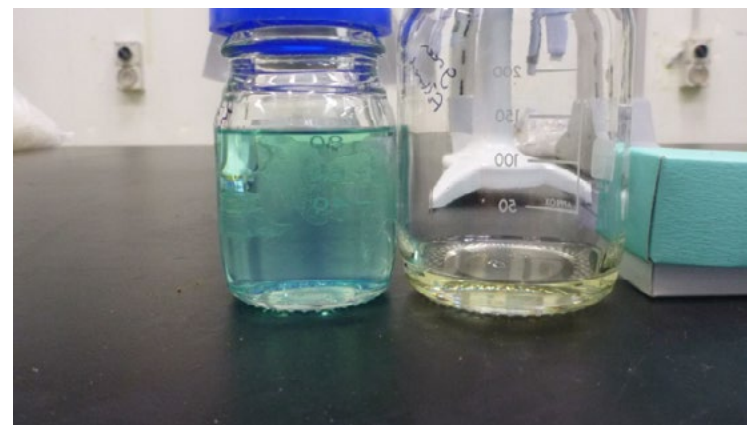
Figure: 15 – Green dye before (left) and after (right) filtration.
