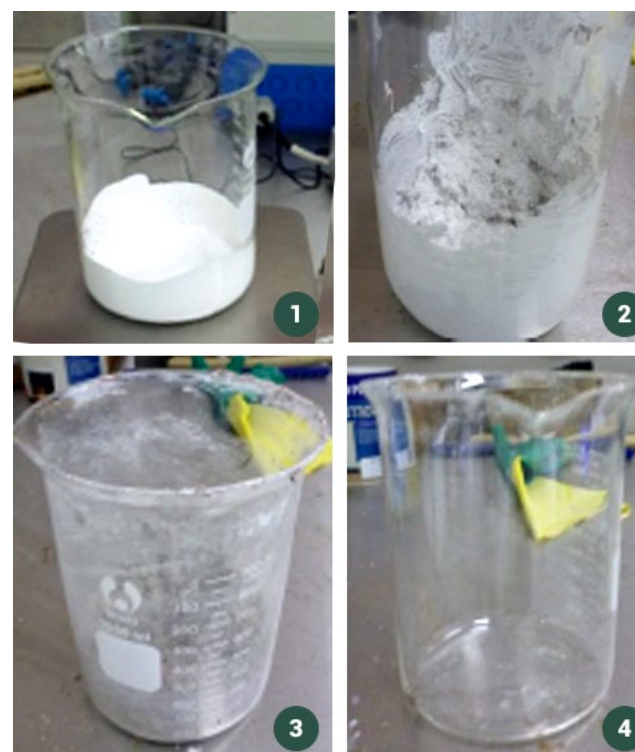
Figure: 18 – Step-by-step paint absorption process
